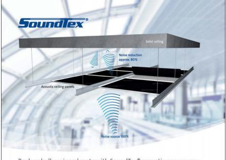
Replace bulky mineral mats with SoundTex® acoustic nonwovens - an ultra-thin textile engineered to absorb sound in the busiest environments.
