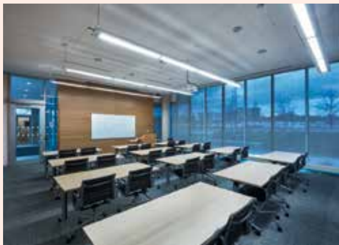
The ceiling panels selected for the project have an NRC as high as 0.90 to optimize acoustics, which can help increase speech intelligibility and dampen ambient noise.
