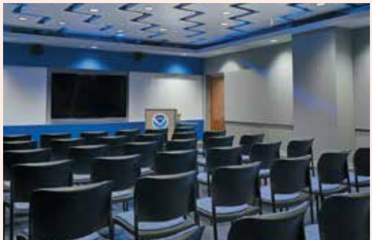
To create the effect of "lightning bolts," two-by-four metal ceiling panels were installed diagonally across the room in a herringbone pattern.
